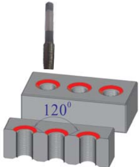
Chamfer with 120° used for tap holes, which reduce the loss of threads.
